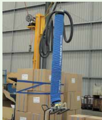
Vacuum lift is used to palletise finished product.
