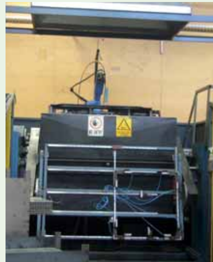
Rotating jigs handle and align the parts being welded.
