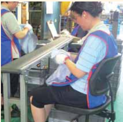
This workstation keeps the materials in the best working zone for the worker.
