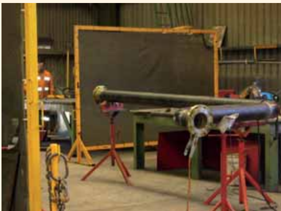
This adjustable stand helps keep the task within the best working zone.
