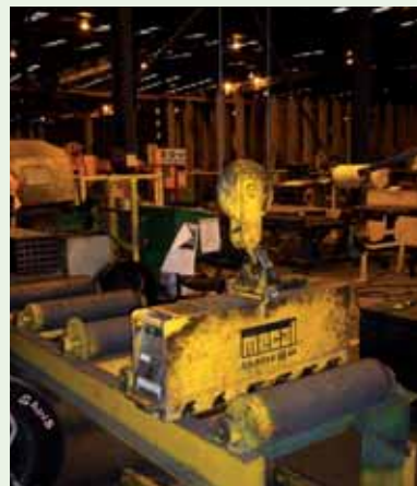
A magnetic lifter is used to transfer product off machinery.
