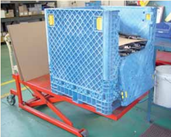
Drop down side improves access for the worker.
