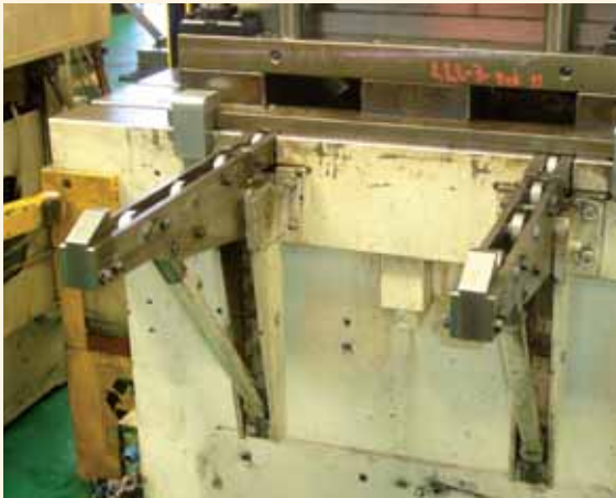
Press with die/tool positioning guides.
