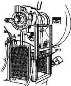
Gates are, in many instances, designed to be operated with each machine cycle. If the gate is not permitted to descend to the fully closed position, the press will not function. Another potential application of this type of guard is where the gate is a component of a perimeter safeguarding system. Here the gate may provide protection not only to the operator but to pedestrian traffic as well. There are two types of gate functions:
