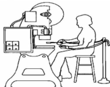
**3. Safety Trip Controls:** These devices provide a quick means for deactivating the machine in an emergency situation.
