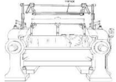
**Safety tripwire cables** are located around the perimeter of or near the danger area. The operator must be able to reach the cable with either hand to stop the machine. All of these tripwires, rods or other safety devices must be manually reset to restart the machine.
