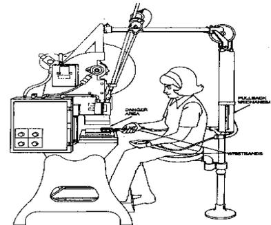
The **restraint (holdout)** device uses cables or straps that are attached to the operator's hands and a fixed point. The cables or straps must be adjusted to let the operator's hands travel within a predetermined safe area. There is no extending or retracting action involved. Consequently, hand-feeding tools are often necessary if the operation involves placing material into the danger area.
