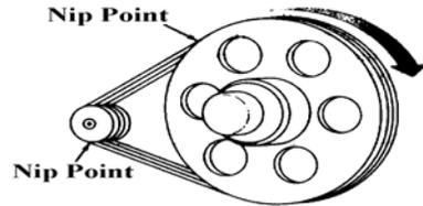
Rotating and tangentially moving parts
