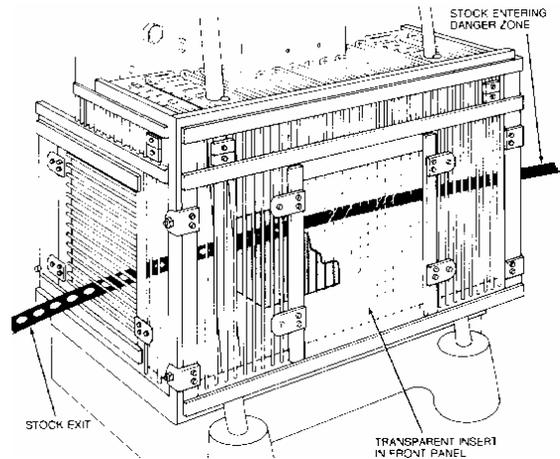
**Interlocked Guards:** When this type of guard is opened or removed, the tripping mechanism and/or power automatically shuts off or disengages, and the machine cannot cycle or be started until the guard is back in place.
